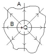
The figure shows two surfaces A and B of different shapes and sizes enclosing a given charge +Q.
